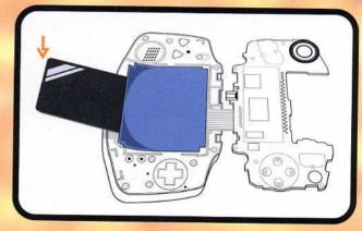
**Notes:** To remove the LCD, position the plastic card under the edge of the LCD and gently pry it off of the front casing. You may have to push back some of the gray cushioning on the LCD to make room for the plastic card.
