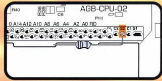
Solder one end of the resistor included with the kit to the lead labeled 'S2' on the GBA mainboard a shown in the above diagram. Position the resistor in the crevice as shown to prevent added internal stress to the LCD when the system is reassembled.
