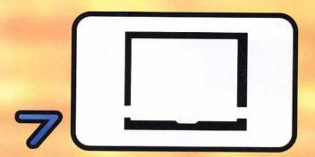
Cut the adhesive cushion as shown. Discard the bottom piece, and replace the upper piece of the cushion into the front casing. Then replace the plastic screen cover onto the front casing (see diagram from Step 12).
