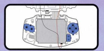
Replace the a/b buttons, start/select buttons, and directional pad. Then reinsert the mainboard into the front casing of the GBA.
