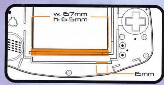
Both sections of plastic, highlighted above, must be cut from the front casing to allow for the After-burner to fit properly. The larger section should be cut entirely through the front casing. The smaller section should only be trimmed down to the surrounding surface (see diagram from Step 12).
