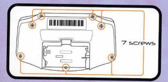
Ensure that there are no batteries or game cartridges in the system. Remove the battery cover. Then remove the six screws from the rear casing of the GBA along with the screw behind the battery cover. Pull the rear casing off of the GBA and set it aside along with the seven screws.
