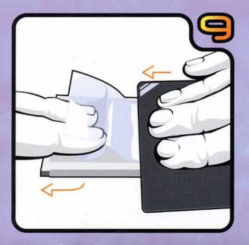
Read the following step in its entirety before continuing: Before moving on, ensure that the LCD surface is completely free of dust and fingerprints. Then laminate the AR film to the LCD surface so that it completely covers the lighter colored area of the LCD. After the film has been applied, remove the release liner from the upper surface of the AR film.
